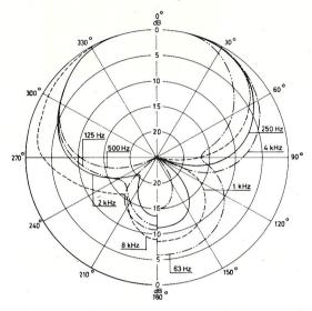
This polar pattern and frequency response curve correspond to typical machine run specifications from a standard M 160.
