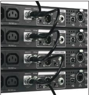
RF distribution ports allow up to 10 receivers to share a single pair of antennas.
